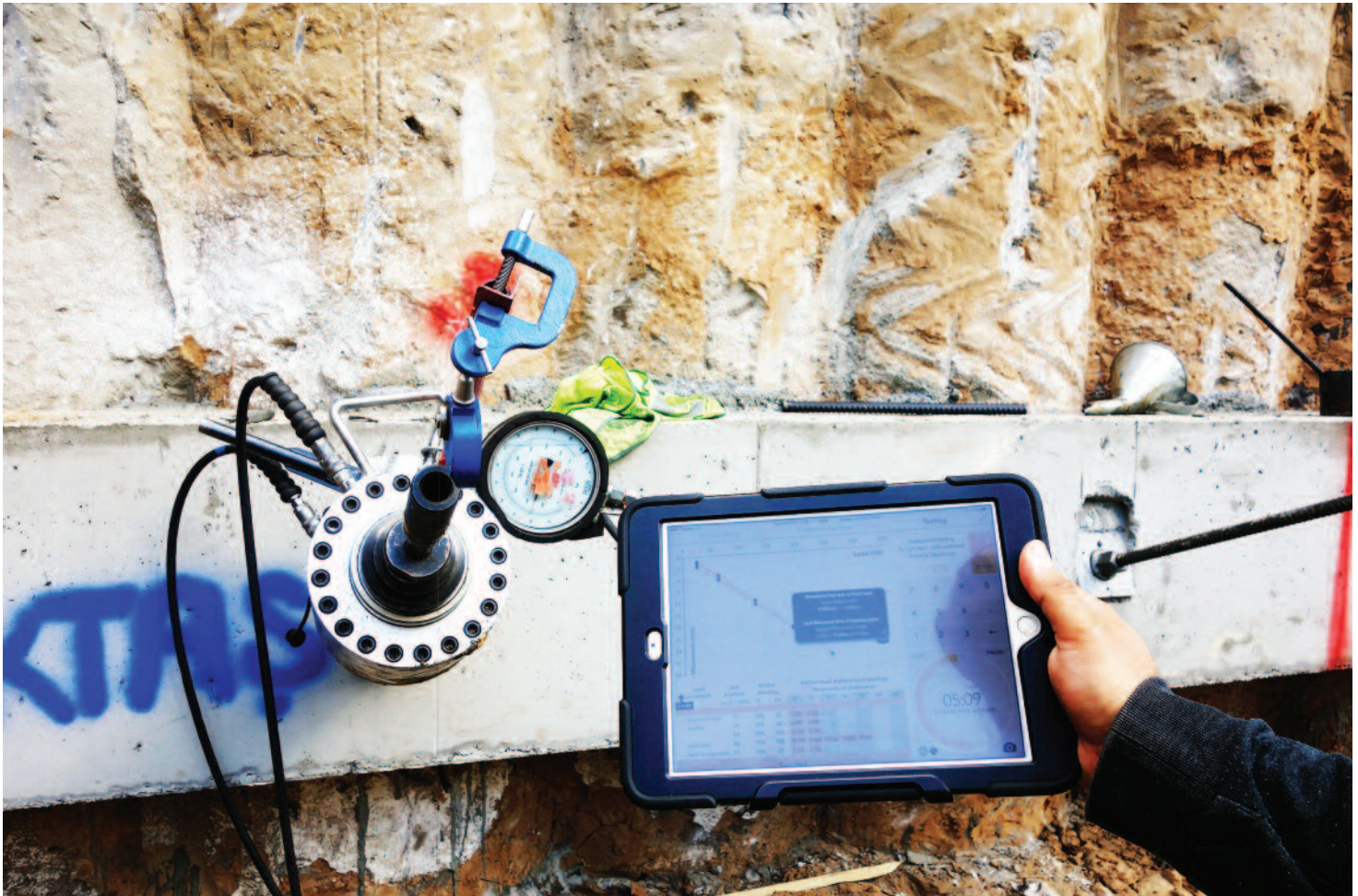
Figure 6 AnchorTest on the field for NOX Project, Moscow.
